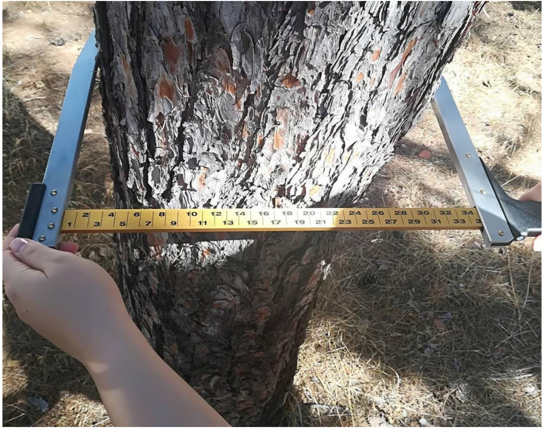
Figure 6. Using a tree caliper for the measurement of DBH.
