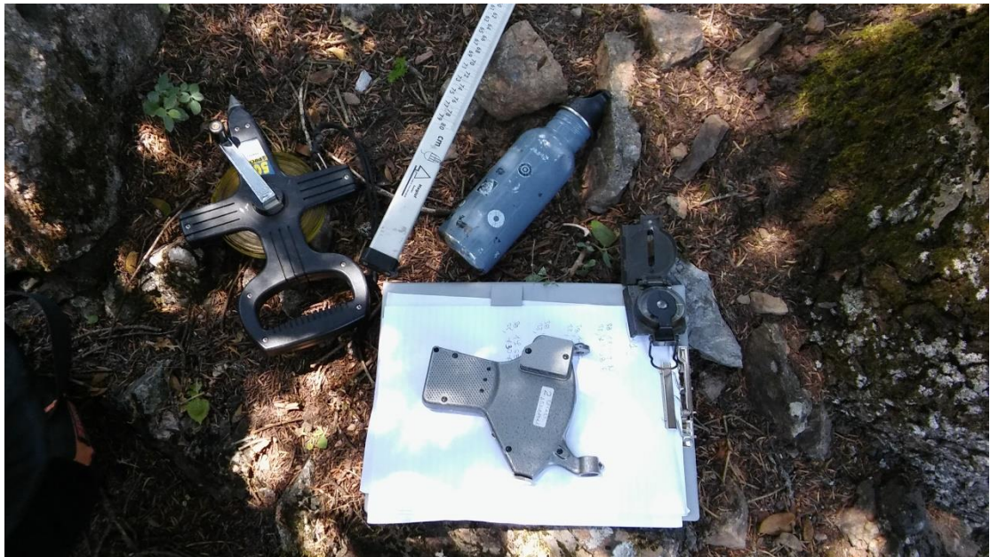
Figure 9. Field work equipment, including measuring tape, tree caliper, clinometer, compass and notepad.
